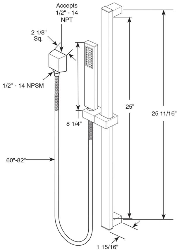
The minimum required water pressure is 0.05 MPa (0.5 bar).
